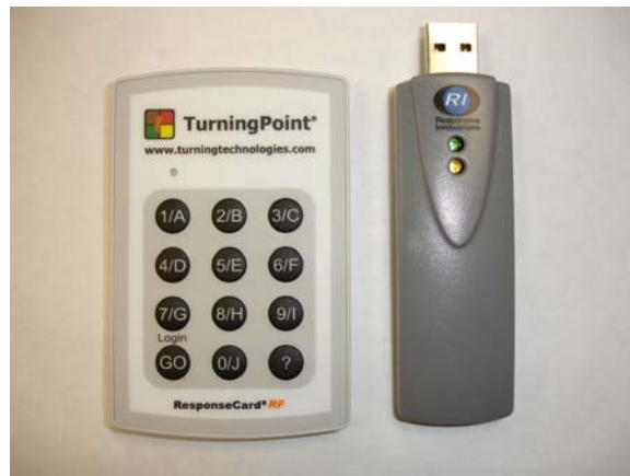
Figure 1. The TurningPoint Audience Response System Response card used by student (left) and receiver used by the instructor (right)
